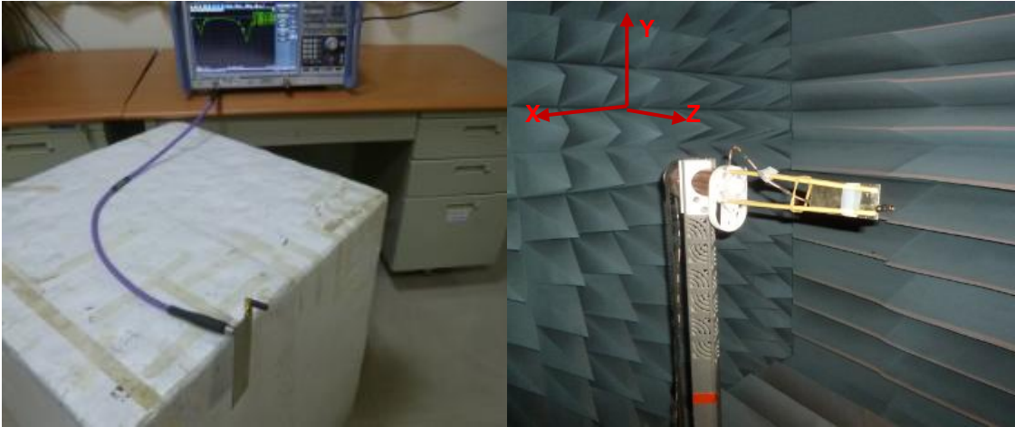
Figure 1. Impedance measurements (left hand) and peak gain, efficiency and radiation pattern measurements (right hand).
